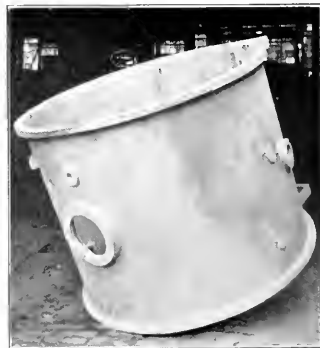
Bronze evaporator shell for 10,000-ton cruiser, 68 inches diameter and height, 5/8-inch walls.
